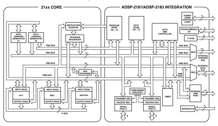
Figure 1. ADSP-2181/ADSP-2183 Block Diagram
